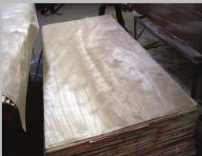
Apply the veneer and go through the second time hot press process
