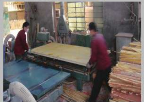
Second time sanding, polishing and cutting into the right size
