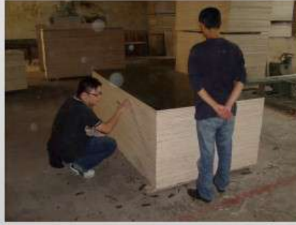
Checking moisture content, size, thickness & veneer surface
