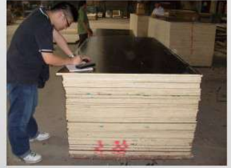
Checking moisture content, size, thickness & veneer surface
